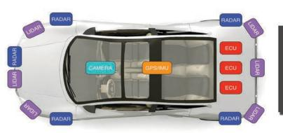
This sample package includes RADAR, LIDAR, a camera, GPS/IMU and ECU. Options, however, are unlimited. We are happy to install sensors to meet your needs. For more information visit www.AutonomyKit.com.
